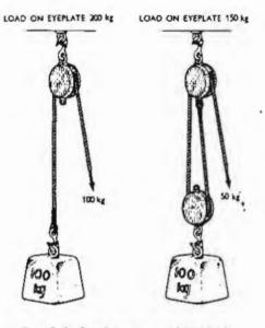
FIG. 8-9. Load on the standing block
