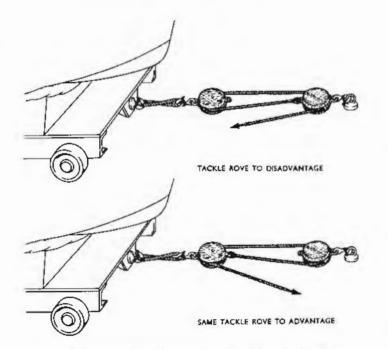
FIG. 8-8. Reeving a tackle to advantage and to disadvantage
